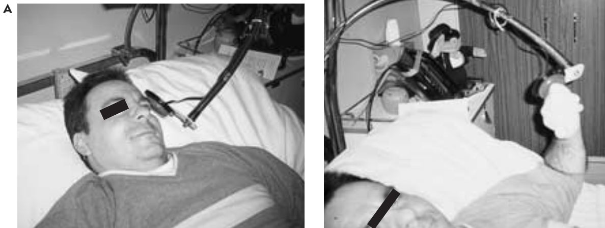
Figure 5.1 (A) A call-button on a flexible support to alert the nurse, controlled by the head. (B) A flexible call-button, hand controlled.
