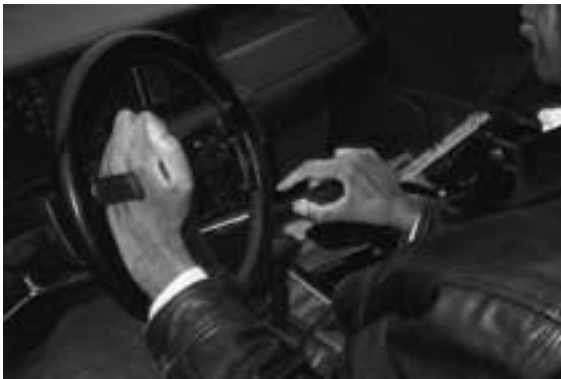
Figure 5.9 Adaptive driving using a fork on the steering wheel and a brake–accelerator lever.
