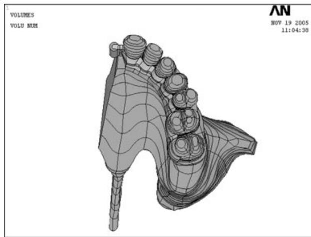
**Fig. 2.** 3D FEM of the lingual guide plane on all the remaining teeth (from central incisor to second molar) with attachment on the mesial surface of the central incisor.
