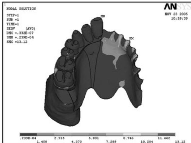
Fig. 4. Stress on the prostheses (model 1).
