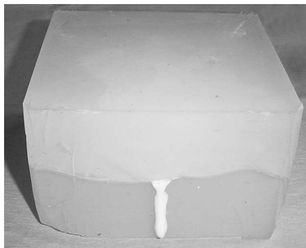
Fig. 1 – Silicone rubber mould in which the polyethylmethacrylate paste was cast. Note the thickness of the mould's walls and the excess material appearing at one of the drain channels.
