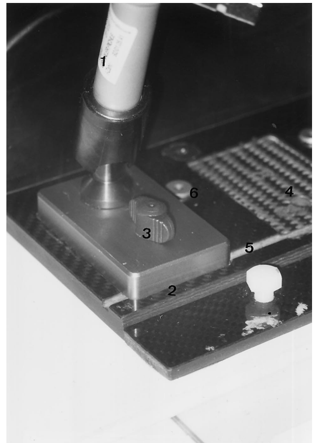
Fig. 6. Base of a hydraulic arm (with patient sticker) (1) attached to the head plate (2) by thumb-screw (3). Also visible on the head plate are an empty impression with threaded bore (4) and a groove for the localization box (5).
