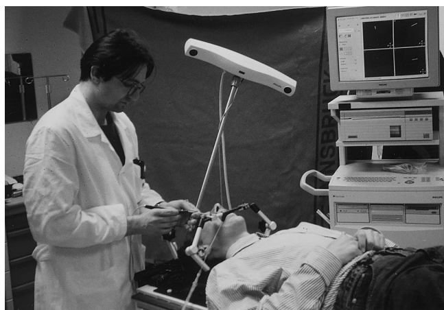
Fig. 7. Setup with subject fixated in VBH head holder with navigation system (Phillips Medical Systems), operator1 (with pointer), operator2 (manning computer) not shown.
