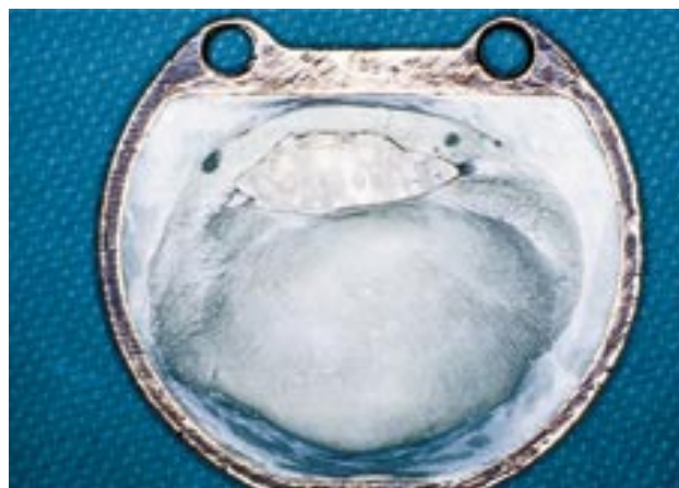
Fig. 5. Invested cast with wax pattern removed after boil-out. Acrylic resin substructure with numerous perforations was fabricated on cast.
