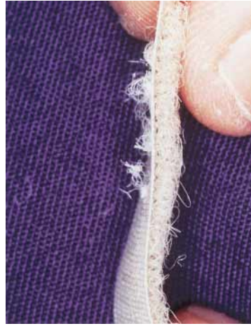
Fig. 5. Loops pulled through backside of Velcro strip.
