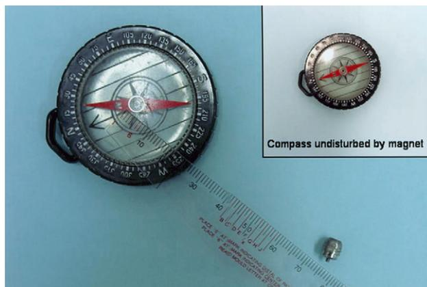
**Fig. 7.** Closed-field magnet with attached keeper showed deflective effect on compass at distance of 75 mm. Photograph shows how compass needle has moved from its resting position of true north.
